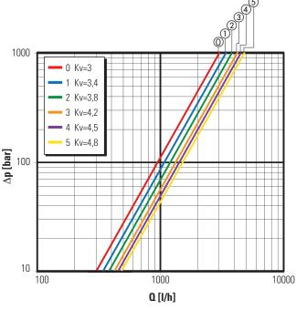
(0)....(5) Position adjusting valve and by-pass Performance detected at -2K
